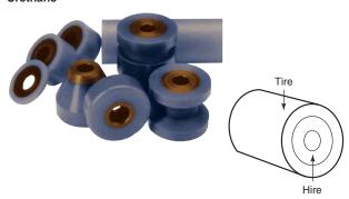
Made from K-prene™ urethane. Low cost alternative for wheels, casters, rollers, sheaves, etc. Blue outer tire (90A durometer) is bonded to a brown hub (75D durometer), resulting in a hard anti-friction bearing with a softer outer tire. Can serve as a bearing in some applications. Comes in 12" and 24" lengths. Cut to fit your application.
