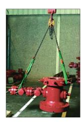
The most easily adjustable and versatile chain sling available. Ideal for machine shop or maintenance departments. Made with grade 80 alloy chain. Proof tested and certified to comply with OSHA.
