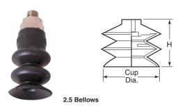
Flat cup is excellent for holding flat, flexible materials without deformation. Bellows cup is excellent for concave and convex shapes such as balls, bottles, or pipe. Evens out variances of machinery and height of objects. Can attach to surfaces which are non-perpendicular. Flat cups are neoprene-chloroprene. Bellows cups are nitrile, which have good oil and abrasion resistance and is good for general purpose use. Use in temperatures to 275 degree Fahrenheit.
