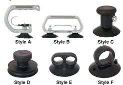
Non-porous materials are easily handled with these vacuum lifters. Styles A, B and C have valve releases to break vacuum. Styles D, E and F are constructed without metal parts and have tabs on the cups to break the vacuum, except A1230-1 which has no tabs.
