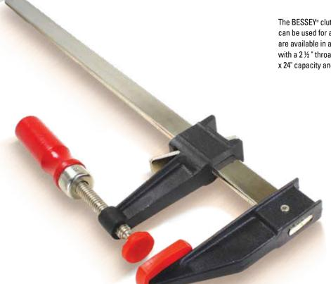
The BESSEY® clutch style clamps are a popular regular duty clamp that can be used for a wide range of projects. These economical clamps are available in a wide range of sizes starting with the GSCC2.506 with a 2 ½ " throat x 6 " capacity up to the GSCC5.024 with a 5" throat x 24" capacity and, a range of clamping force from 600 to 1200 lbs.
