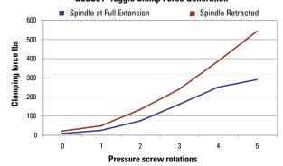
Clamping height: 30mm. Pressure screw set initially to lowest clamp force (0) then 1 full rotation for each measurement point.
