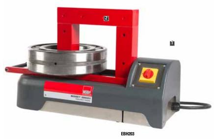
Proper bearing installation is essential to maximum bearing life. By heating prior to installation, the bearing expands and slides easily onto the shaft. Magnetic induction is a safe, efficient method that heats bearings evenly and quickly.
