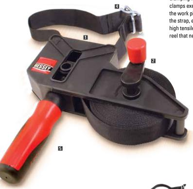
Clamping large or odd shapes with straps is not new; however, most strap clamps exert force (pull) in only one direction which can easily distort/skew the work piece. BESSEY®'s VAS-23 is different, it pulls equally on both ends of the strap, eliminating the chance of skewing your work piece to one side. The high tensile woven polyester strap is extremely strong with a built-in take up reel that neatly stores the excess strap; eliminating a potential tripping hazard.
