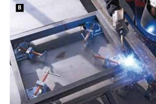
Check out WSM Welders' angle clamps in action!
