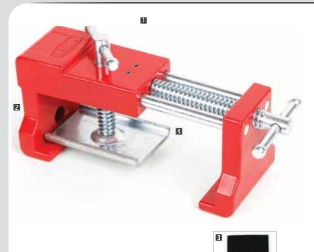
The cabinetry clamp is designed to combine the multiple steps of face frame cabinet installation into one easy process. Face frame stiles can be tightened, aligned, pre-drilled and fastened while the clamp is in place. The clamp holds the individual cabinet edges together while also keeping the faces along the joint flush.
