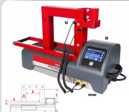
Proper bearing installation is essential to maximum bearing life. By heating prior to installation, the bearing expands and slides easily onto the shaft. Magnetic induction is a safe and efficient method of generating heat to expand bearings for installation. No open flame or hot oil to worry about. Magnetic induction heats bearings evenly and quicker than hot plates.
